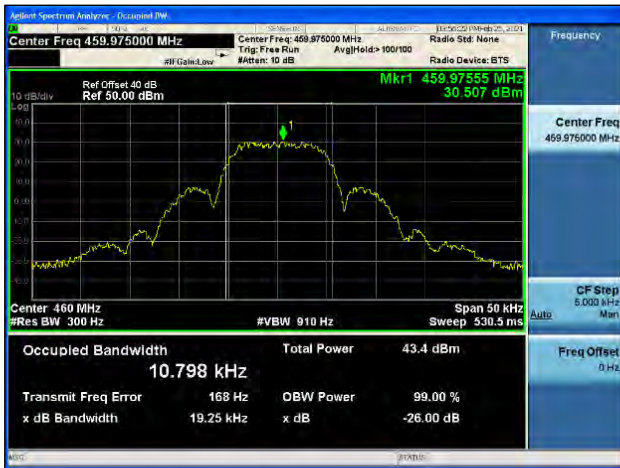
Plot 8-414: OBW 99%, UHF, 459.9750 MHz, WB 2 FSK
