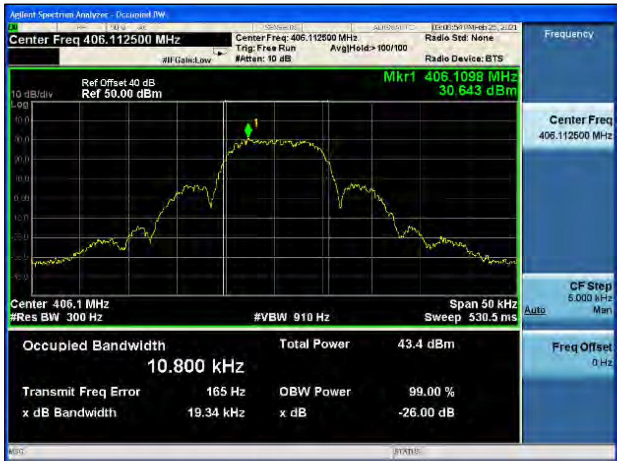
Plot 8-372: OBW 99%, UHF, 406.1125 MHz, WB 2 FSK
