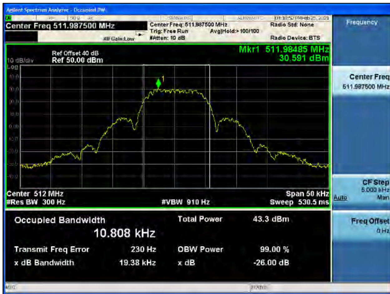
Plot 8-426: OBW 99%, UHF, 511.9875 MHz, WB 2 FSK
