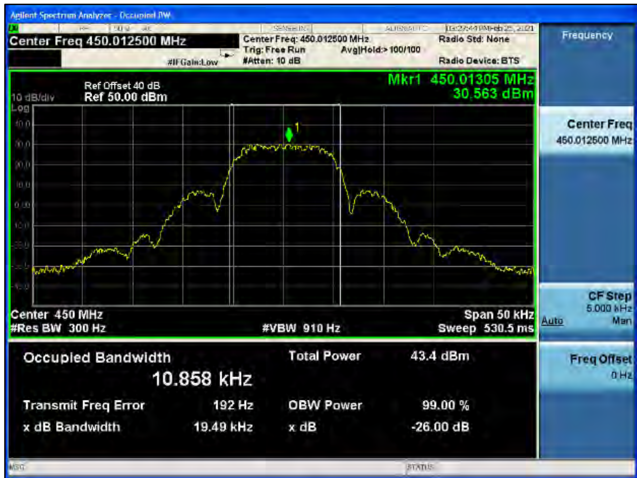
Plot 8-390: OBW 99%, UHF, 450.0125 MHz, WB 2 FSK
