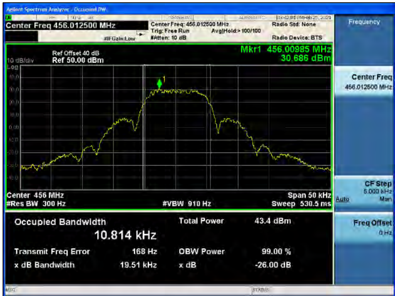
Plot 8-402: OBW 99%, UHF, 456.0125 MHz, WB 2 FSK
