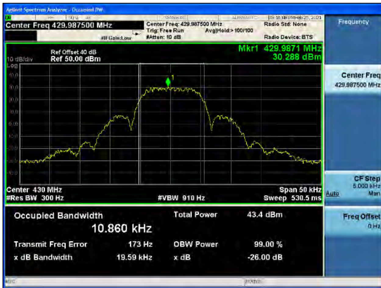
Plot 8-384: OBW 99%, UHF, 429.9875 MHz, WB 2 FSK
