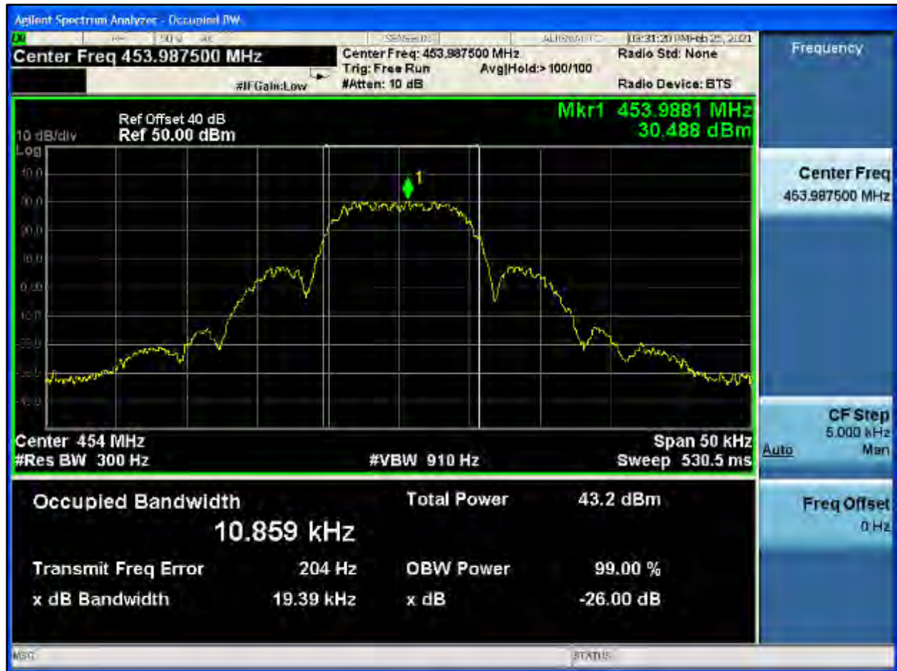
Plot 8-396: OBW 99%, UHF, 453.9875 MHz, WB 2 FSK
