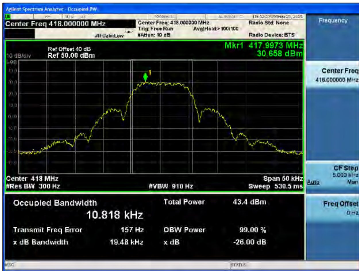
Plot 8-378: OBW 99%, UHF, 418.0000 MHz, WB 2 FSK
