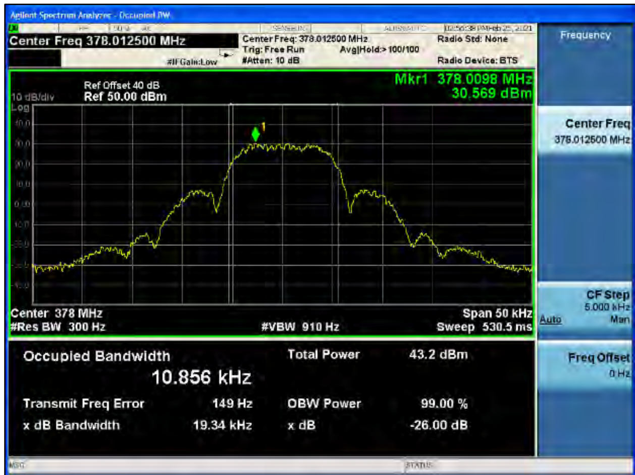
Plot 8-366: OBW 99%, UHF, 378.0125 MHz, WB 2 FSK
