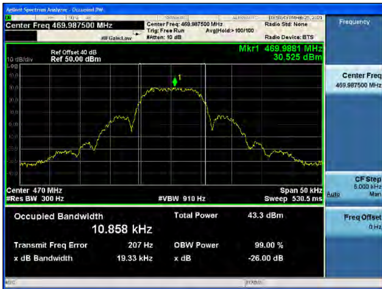
Plot 8-420: OBW 99%, UHF, 469.9875 MHz, WB 2 FSK
