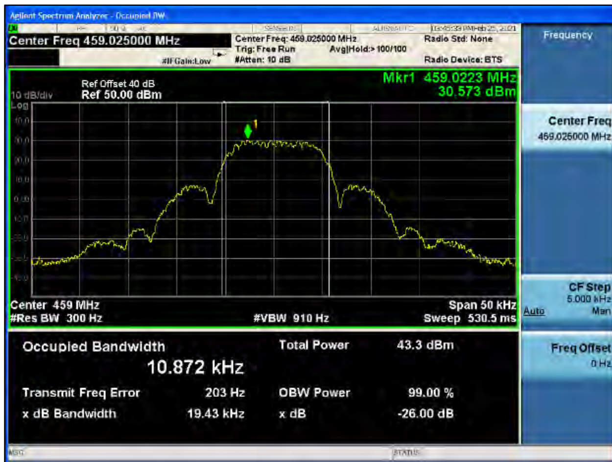
Plot 8-408: OBW 99%, UHF, 459.0250 MHz, WB 2 FSK
