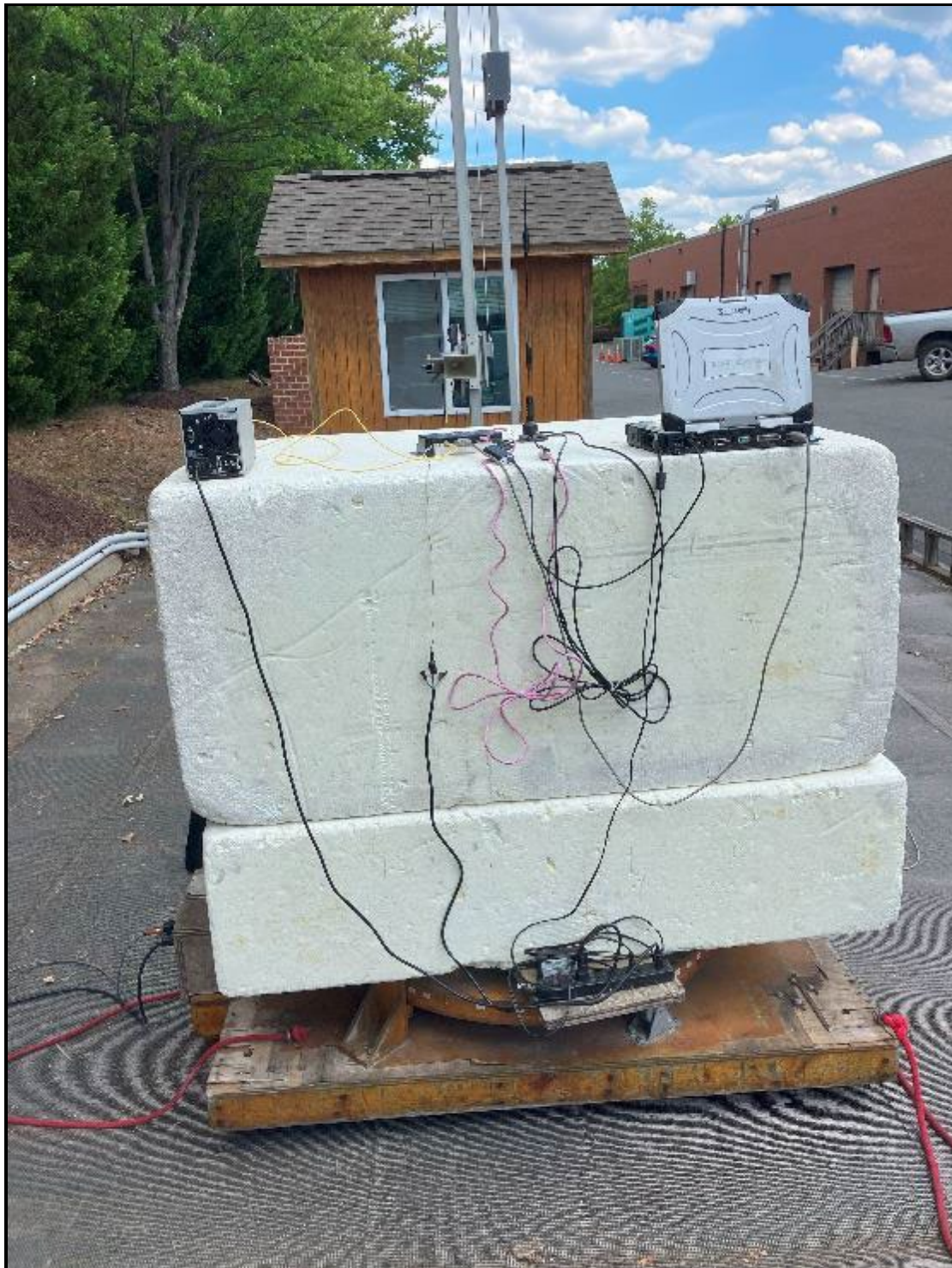
Photograph 2: Radiated Emissions (Spurious/Harmonics) Over 1 GHz, Back View
