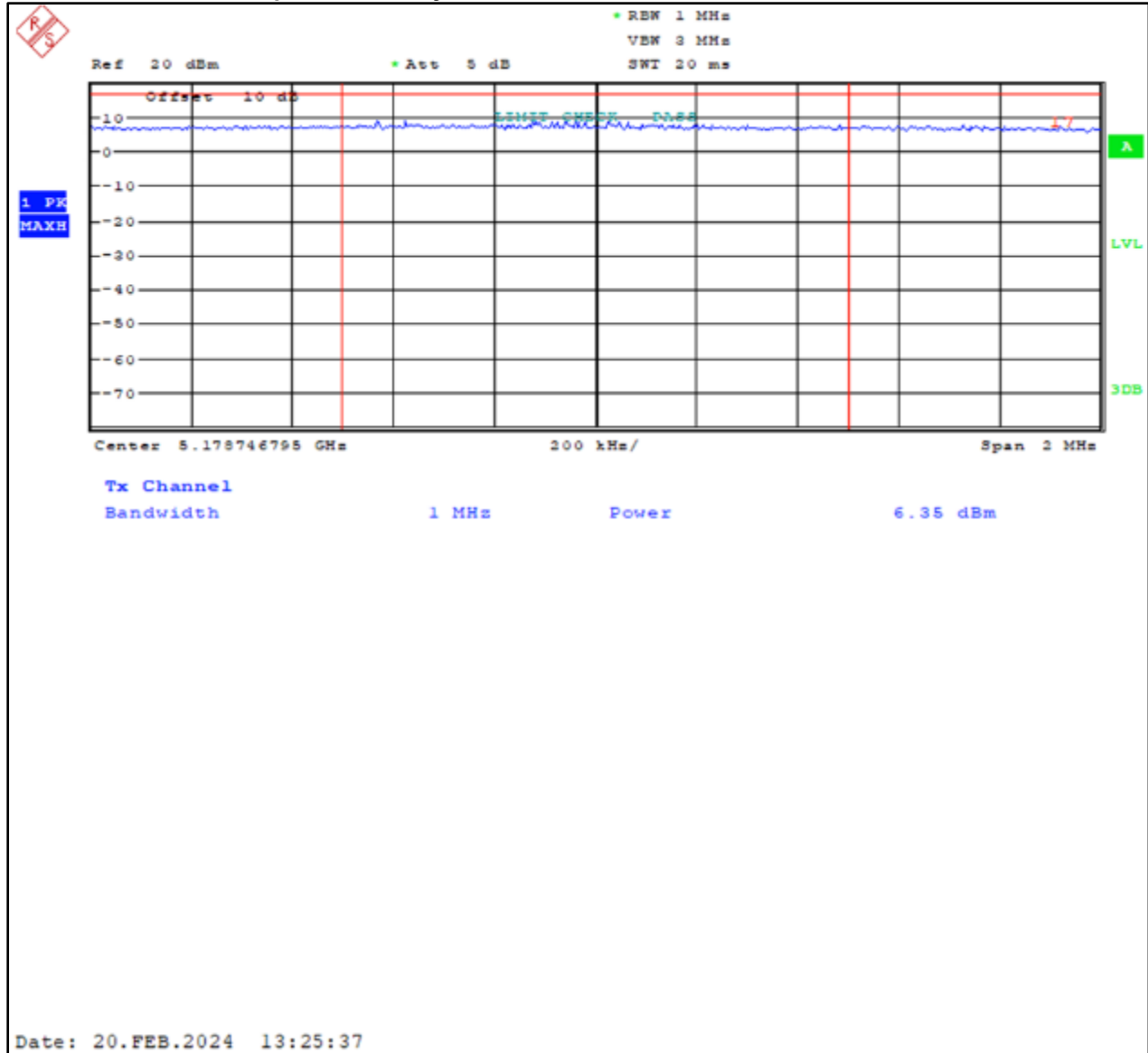
Plot 7-1: Power Spectral Density – 5180 MHz – 802.11a
