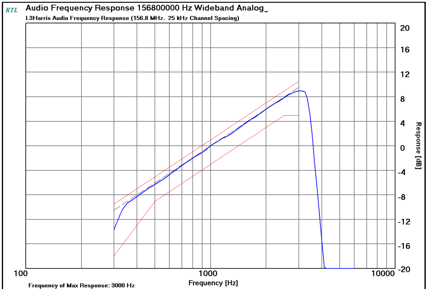
Plot 9-3: Modulation Characteristics - Audio Frequency Response – 156.8000 MHz (WB)
