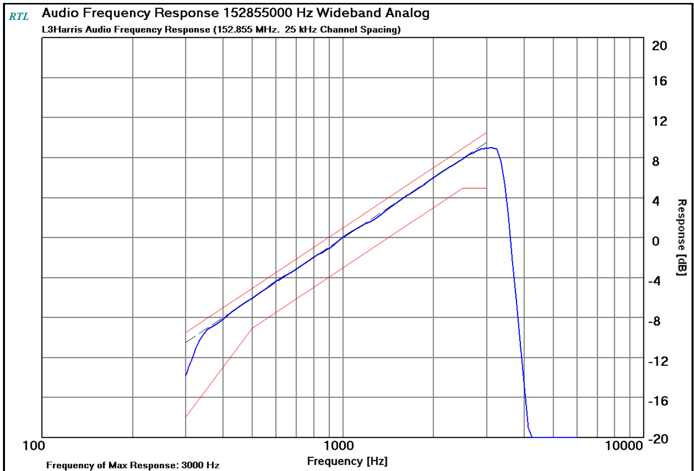
Plot 9-2: Modulation Characteristics - Audio Frequency Response – 152.8550 MHz (WB)
