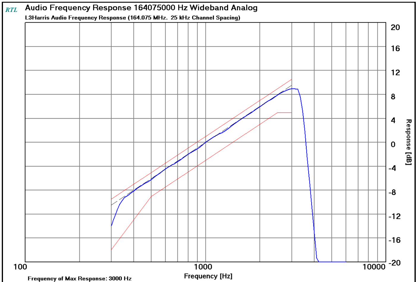
Plot 9-6: Modulation Characteristics - Audio Frequency Response – 164.0750 MHz (WB)
