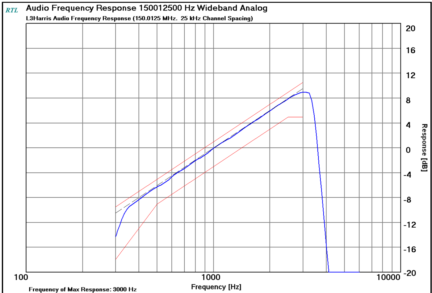
Plot 9-8: Modulation Characteristics - Audio Frequency Response – 150.0125 MHz (WB)
