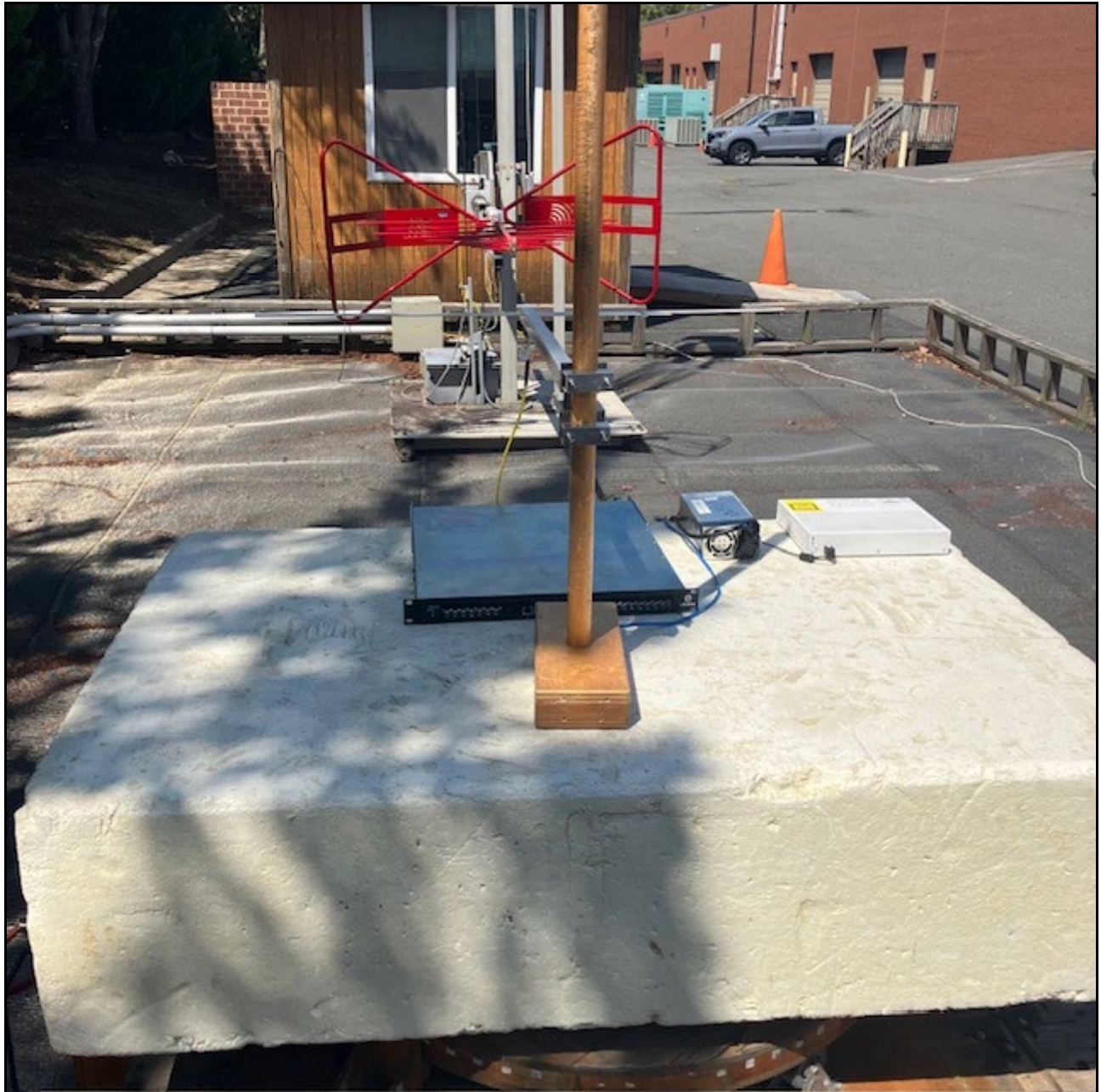
Photograph 1: Radiated Emissions (Spurious/Harmonics) – Front View – Less Than 1 GHz
