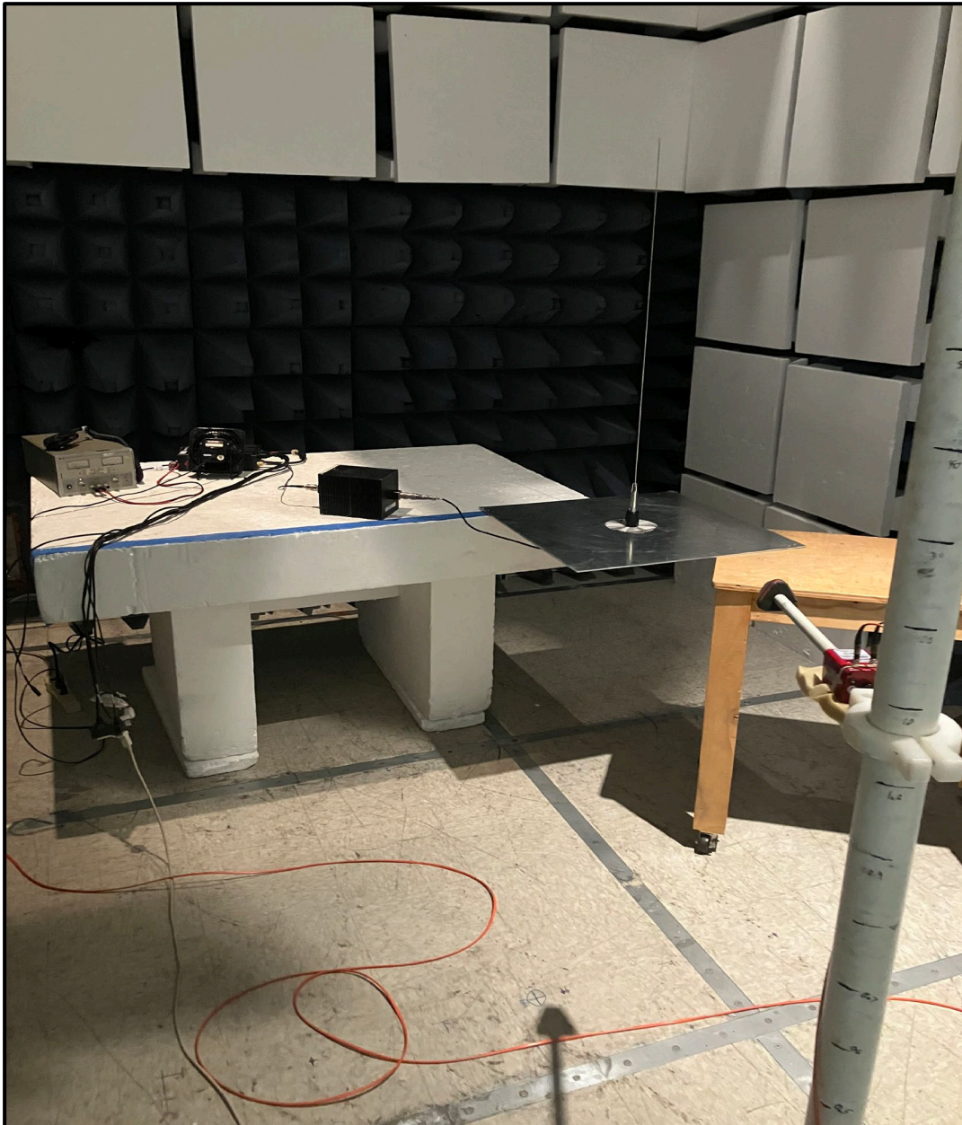
Photograph 2: MPE Setup Using NGP Antenna
