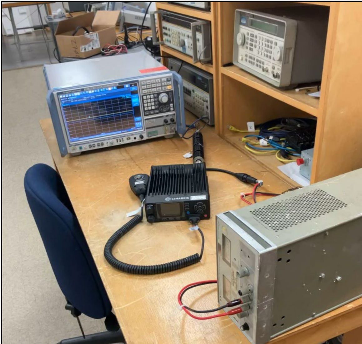
Photograph 7: Conducted Antenna Port Spurious Emissions
