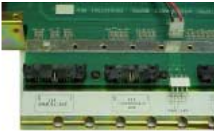
4-Pin POWER, 20-Pin CONV/DSP & 20-Pin SIMULCAST Connectors
