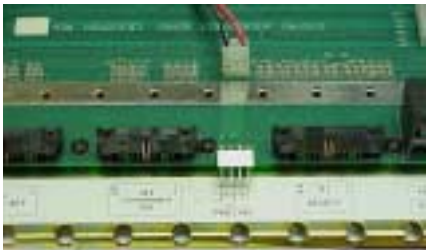
24-Pin EDACS, 4-Pin POWER & 20-Pin CONV/DSP Connectors
