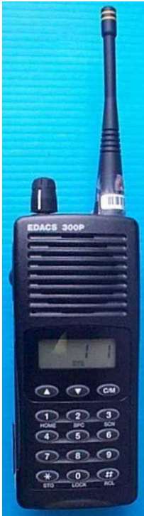
Com-Net Ericsson EDACS 300P FM Portable Radio, with a \lambda/4 antenna and thin battery
