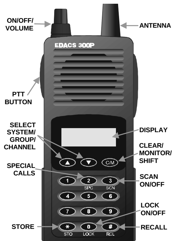
Figure 2. EDACS 300P System Model
