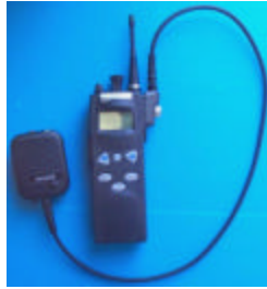
speaker/microphone with antenna port, black, Ericsson, CSA/FM KRY 101 1617/84 (left)
