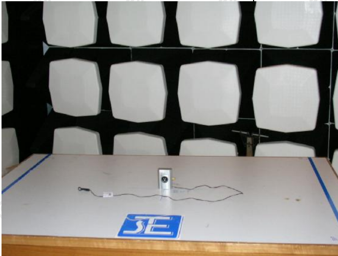
Measurement of Radiated Emission Test Set Up
