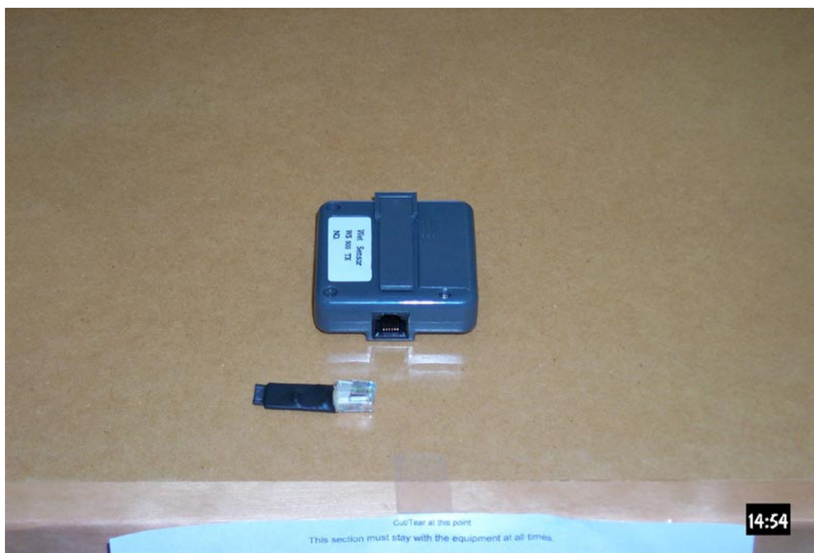
Figure 12 Back of WS900Tx with test probe
