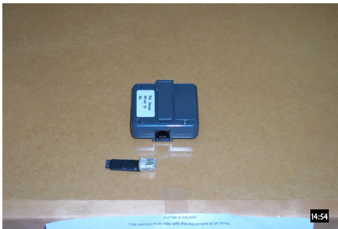
Figure 12 Back of WS900Tx with test probe
