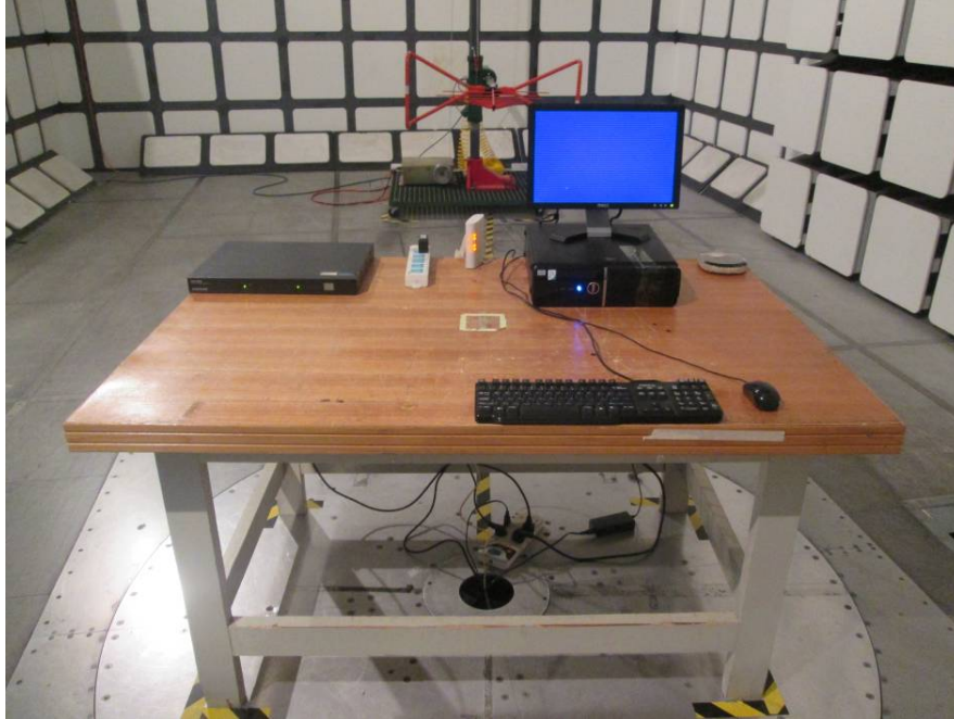
Radiated Emissions – Front View (Below 1 GHz)
