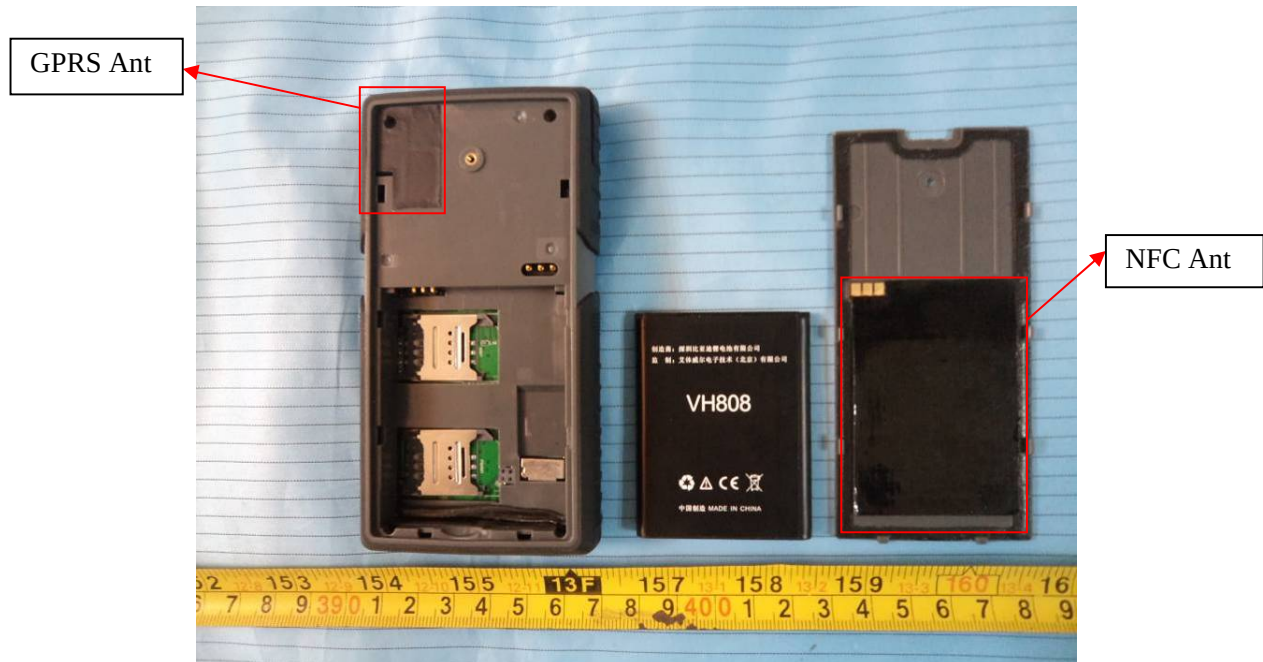
EUT – Battery off View
