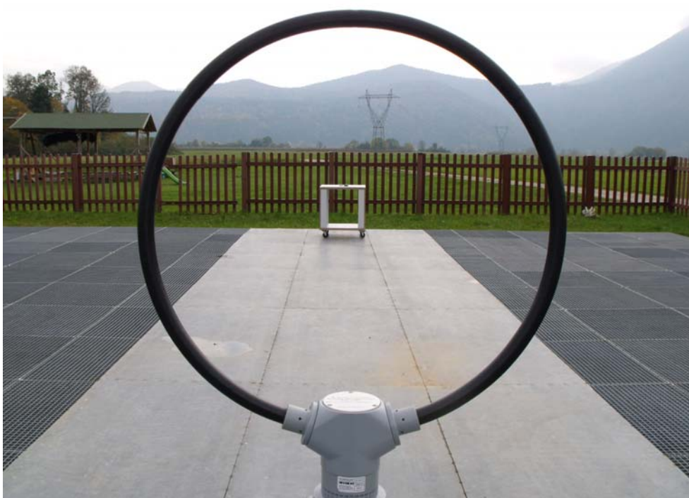
Figure 3: Radiated emission test – under 30 MHz on OATS
