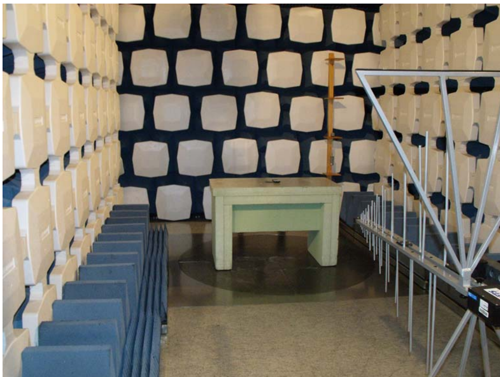
Figure 2: Radiated emission test – over 30 MHz
