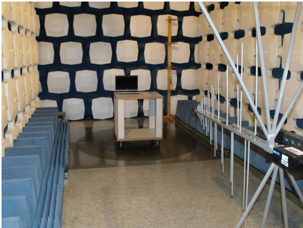
Figure 2: Radiated emission test – over 30 MHz
