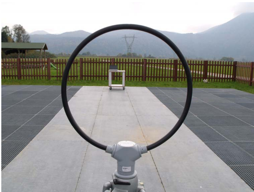
Figure 3: Radiated emission test – under 30 MHz on OATS
