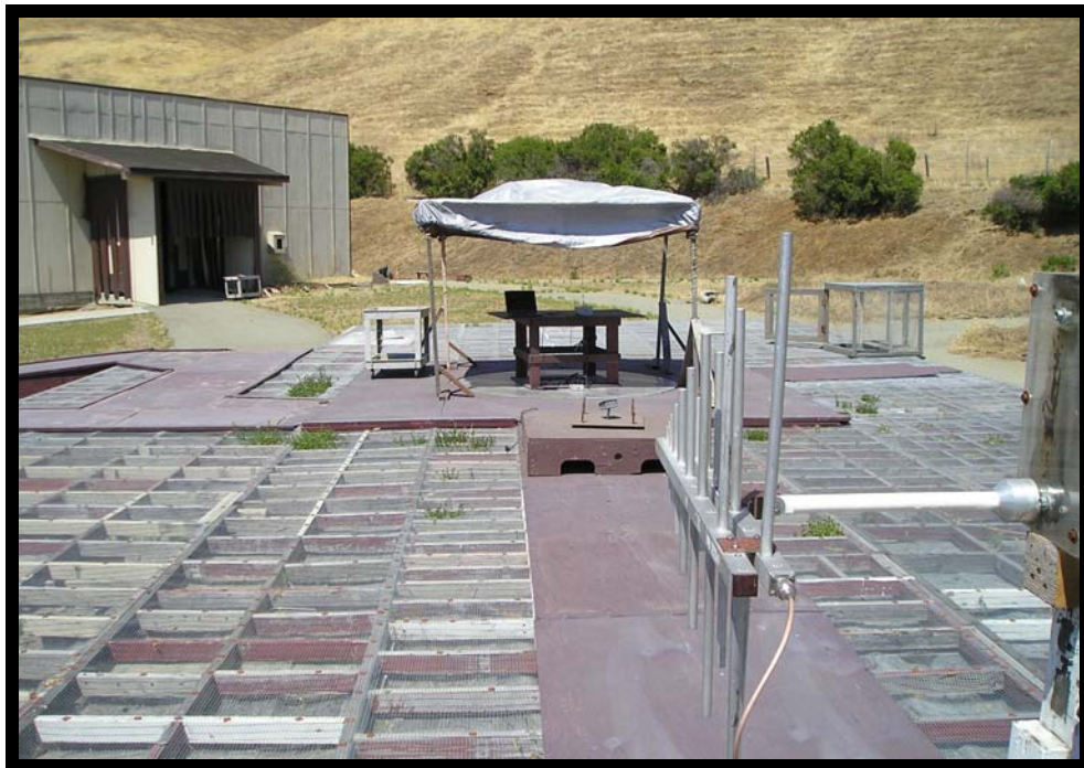
Figure 32: Spurious Emissions Test Setup (Below 1 GHz) Front View
