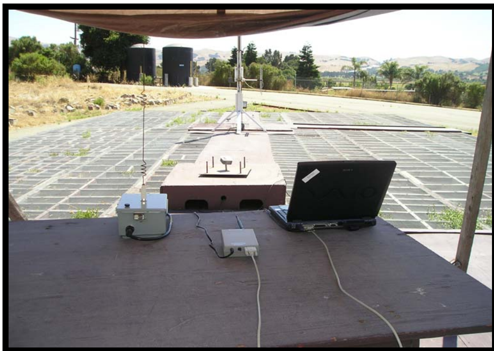
Figure 33 Spurious Emissions Test Setup (Below 1 GHz) Rear View
