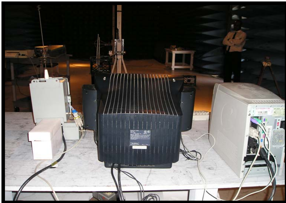
Figure 12: Spurious Emissions Rear View (Above 1 GHz)
