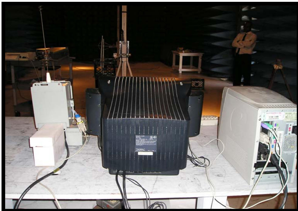
Figure 8: Power Spectral density Test Setup (Rear View)
