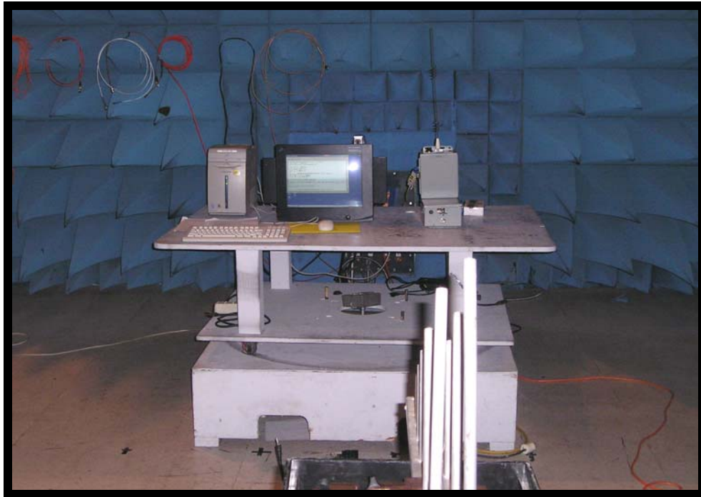
Figure 7: Power Spectral Density Test Setup (Front view)
