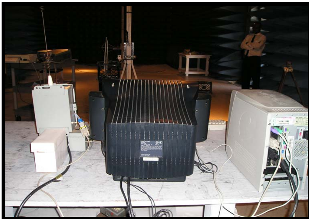
Figure 8: Power Spectral density Test Setup (Rear View)
