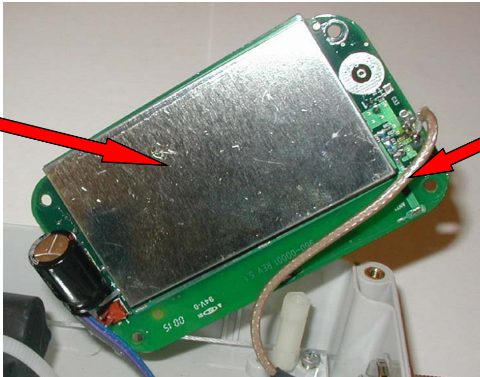
Figure 5 Main-Board RF Section View with Metal Shield Cover
