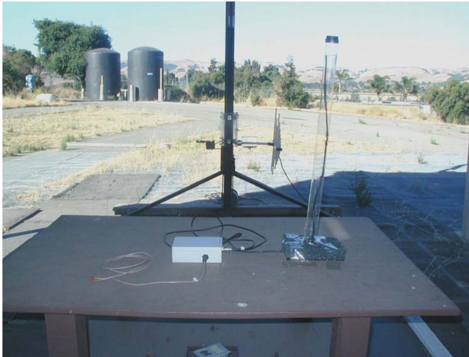
Figure 5 Test Set Up Photos (180 deg) – RF Radiated Measurements
