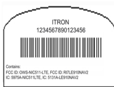
Figure 2 Example of NIC address label for NIC 511-NA1-0313
