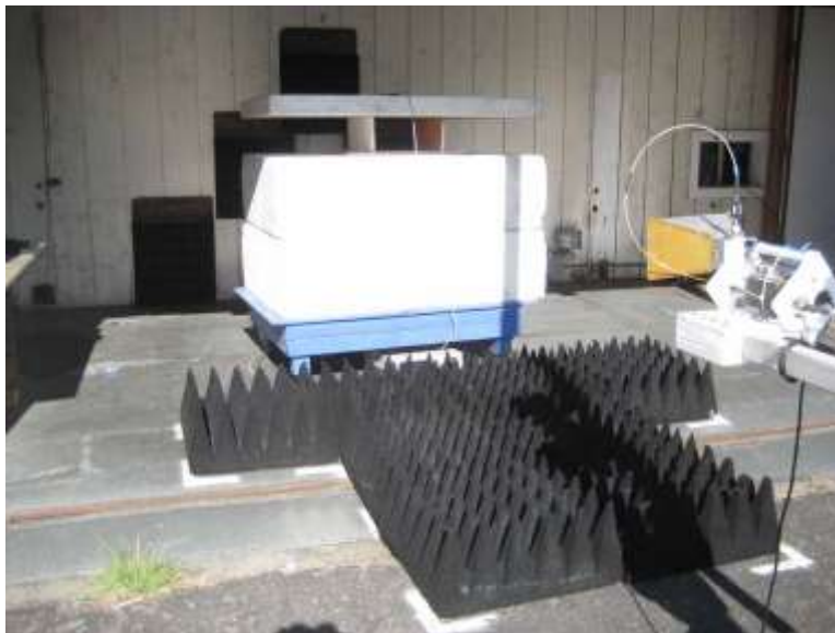
Section 7.12, Above 1GHz Cone placement Test Setup
