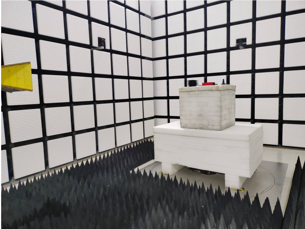
Radiated Emission Above 1GHz View - Adapter Power
