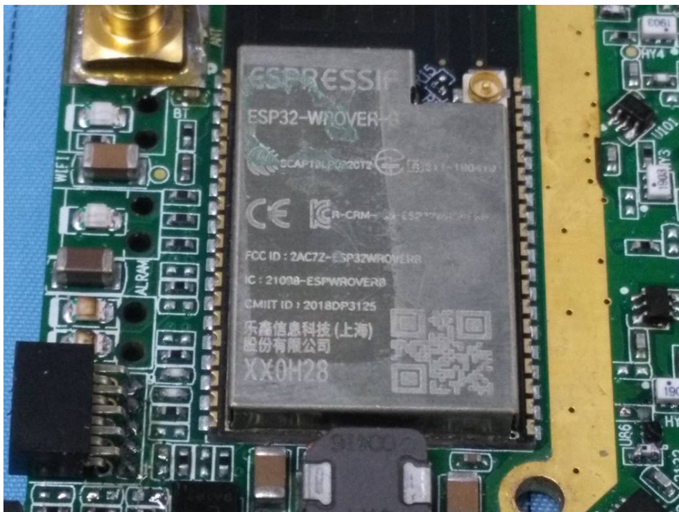
Bluetooth & Wi-Fi Module (FCC ID: 2AC7Z-ESP32WROVERB)
