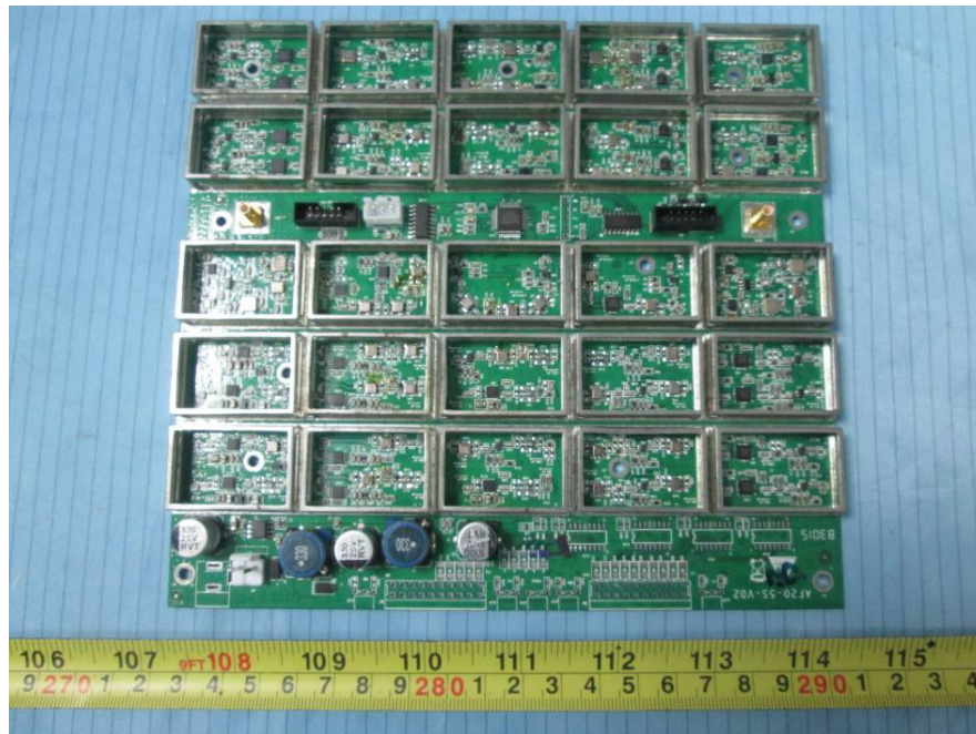
EUT – Main Board 1 Top Shielding off View
