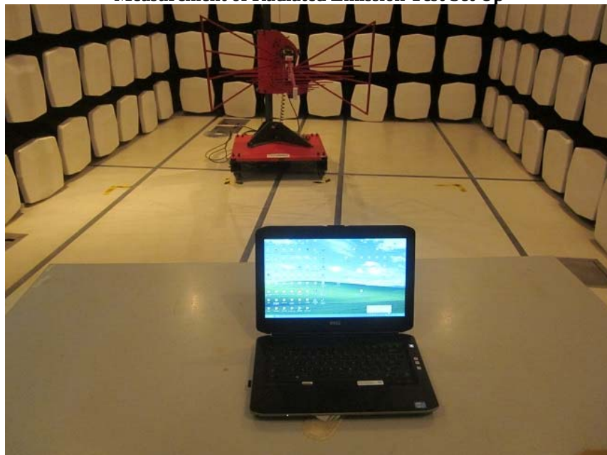
Measurement of Radiated Emission Test Set Up
