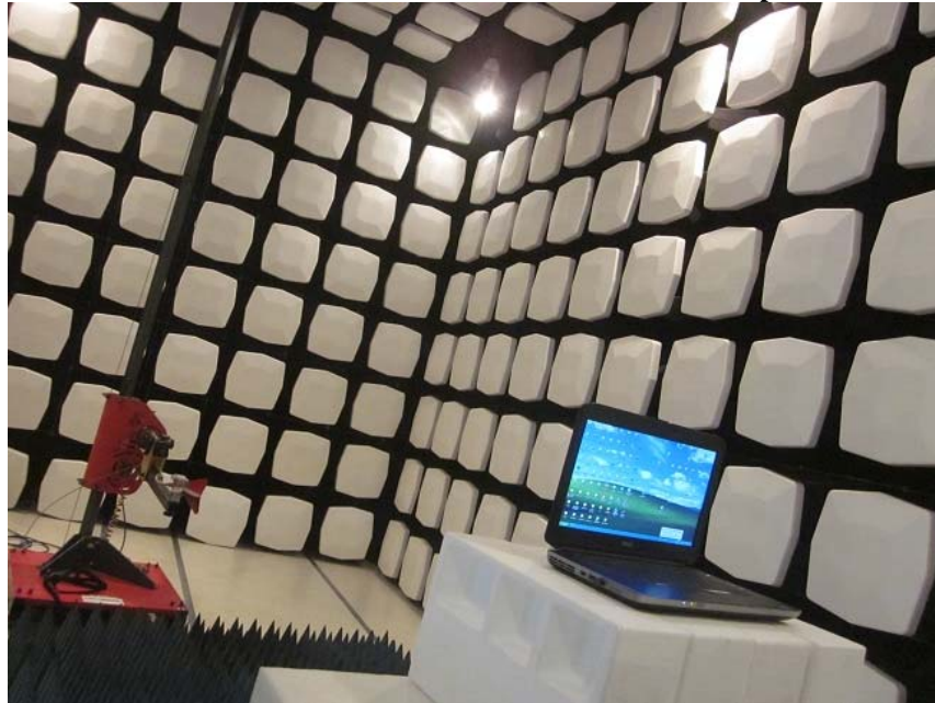
Measurement of Radiated Emission Test Set Up
