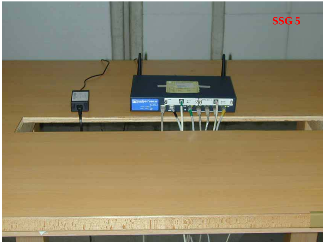
Photo 1: Radiated Emission Test set-up photo
