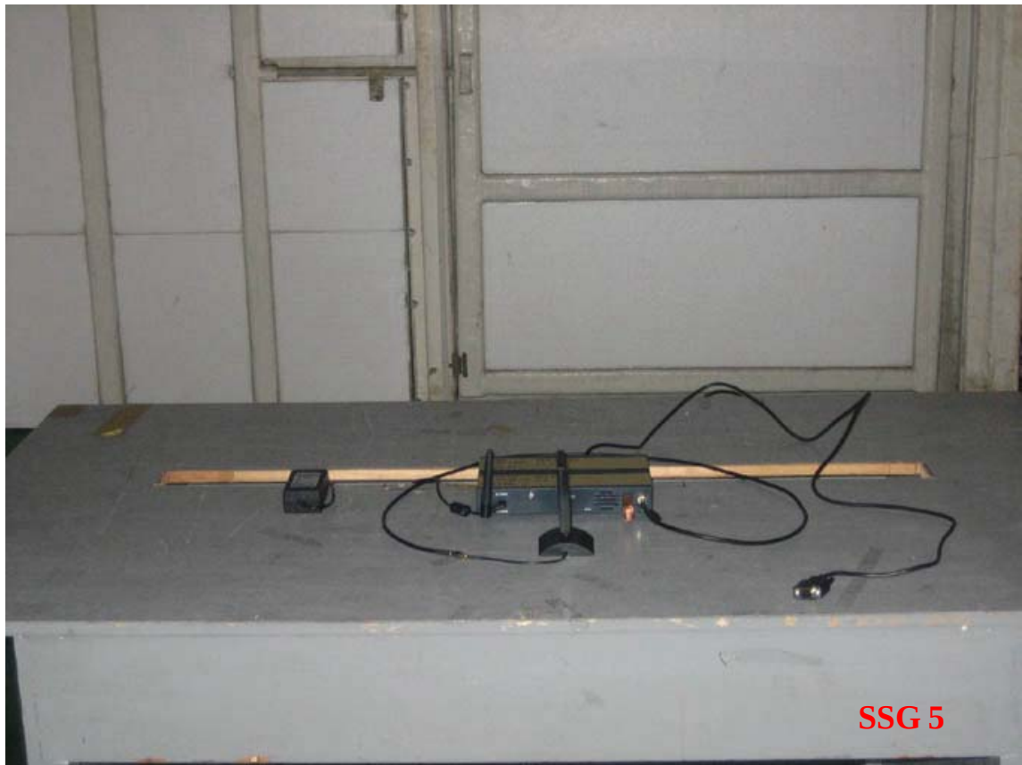
Photo 2: Radiated Emission Test set-up photo
