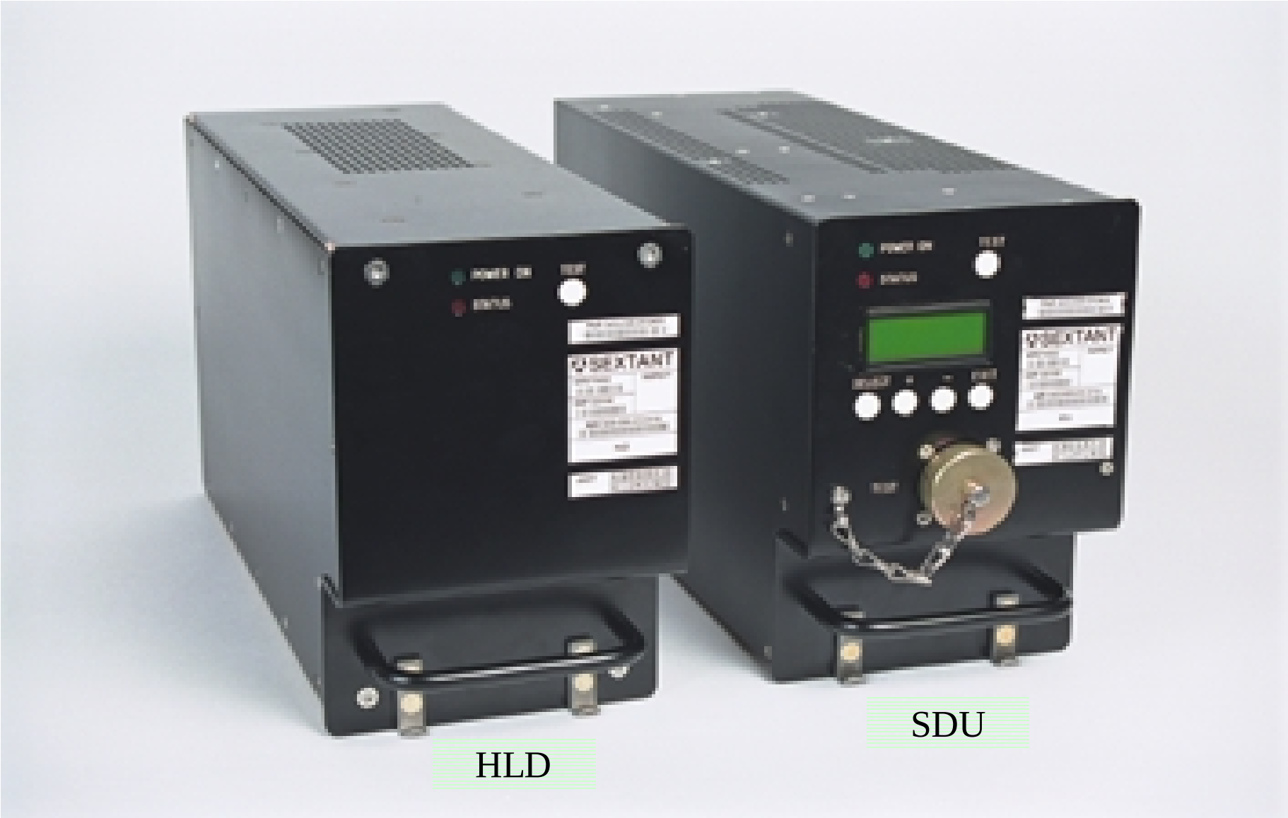
Figure 4: HLD and SDU – External view
