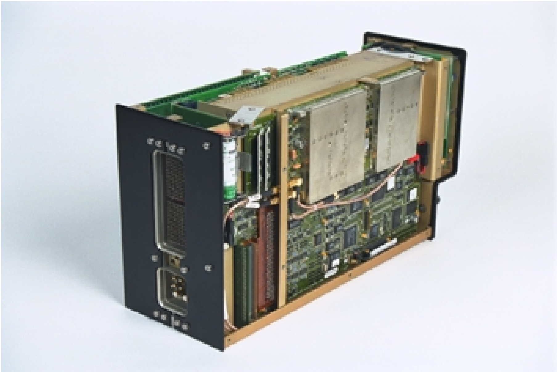
Figure 7: SDU - Internal view
