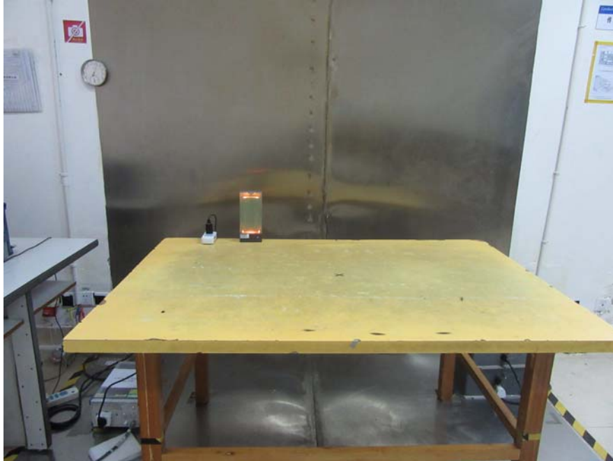
Conducted Emissions – Front View
