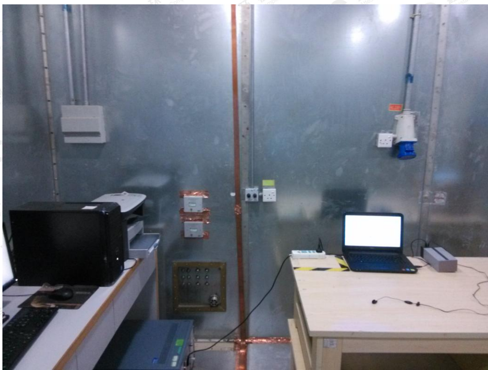
FCC RADIATED EMISSION TEST SETUP
