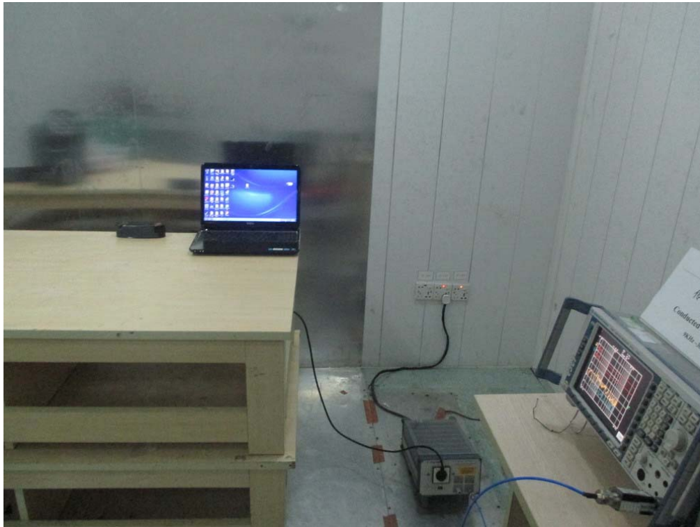
FCC RADIATED EMISSION TEST SETUP
