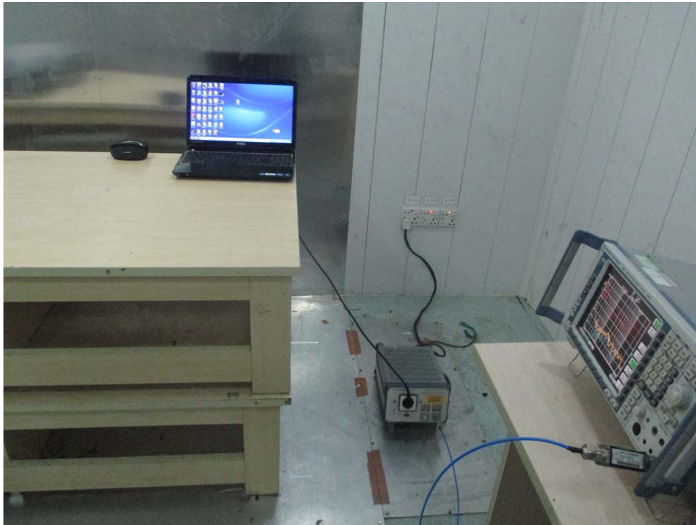
FCC RADIATED EMISSION TEST SETUP
