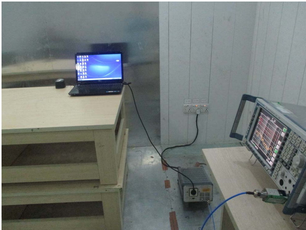
FCC RADIATED EMISSION TEST SETUP
