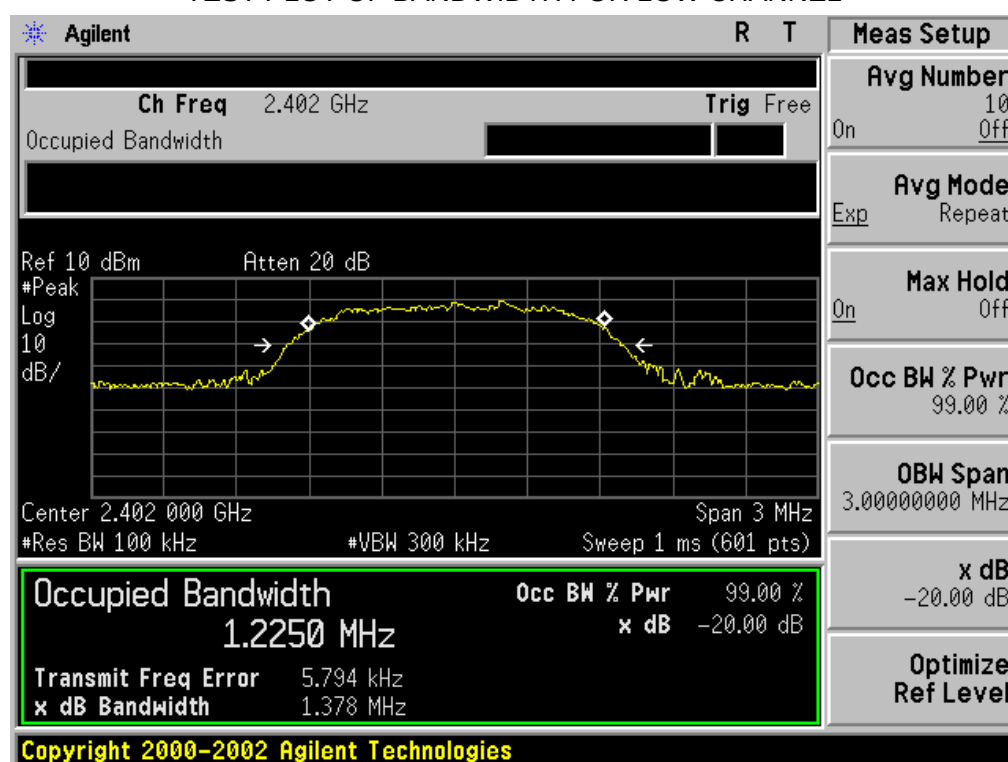
TEST PLOT OF BANDWIDTH FOR LOW CHANNEL
