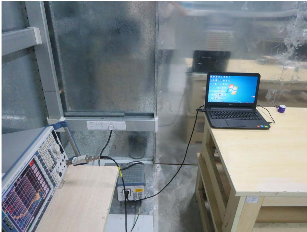
FCC RADIATED EMISSION TEST SETUP
