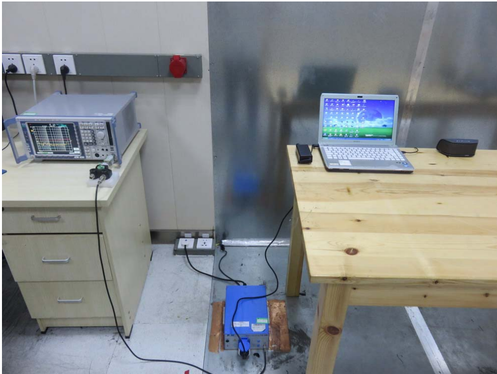
FCC RADIATED EMISSION TEST SETUP
