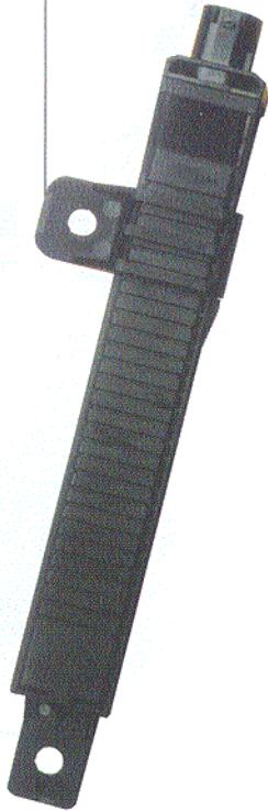
Receiving antenna of the tire pressure monitoring system
