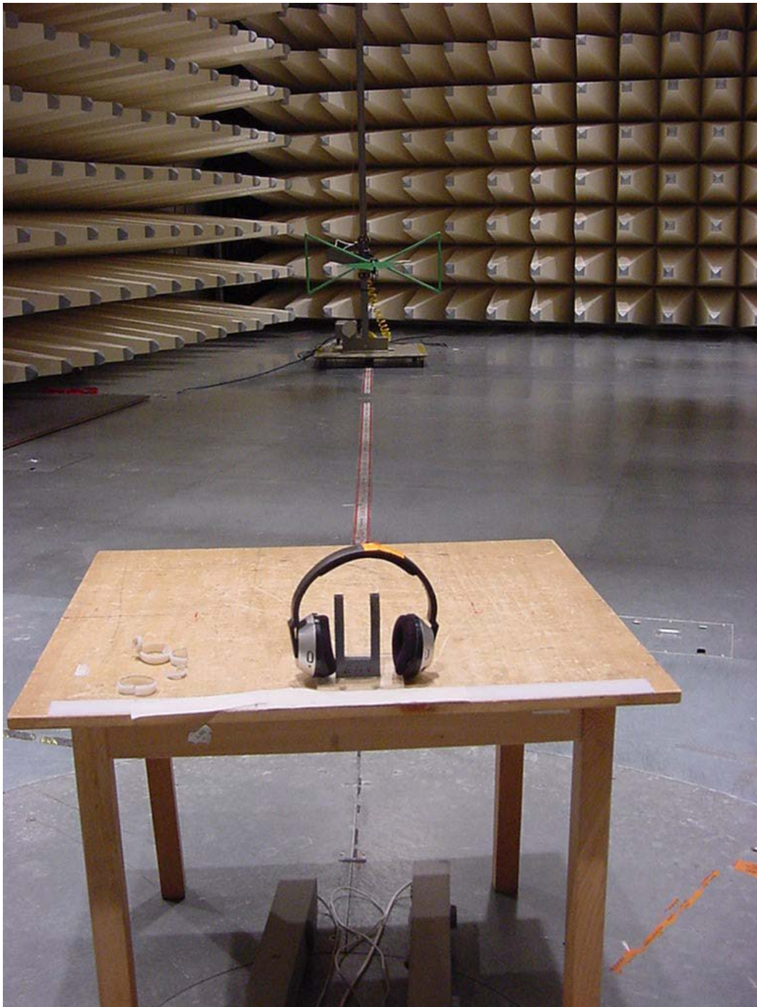
Photo 3 (Radiated Emissions): Rx Test set-up
