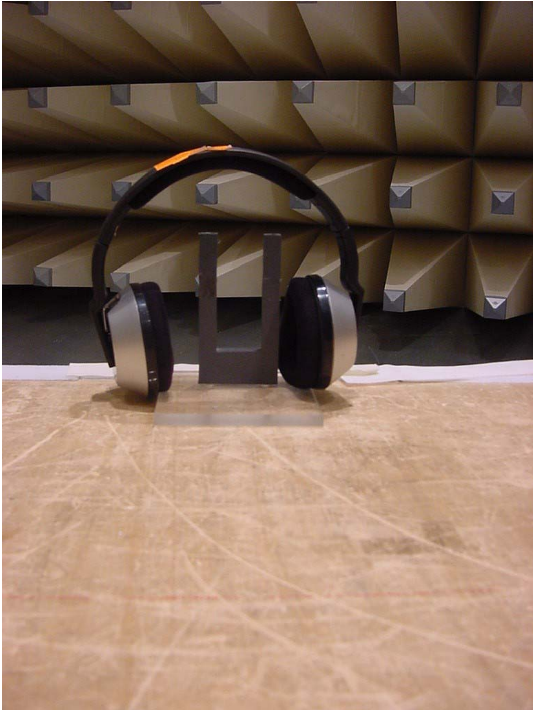
Photo 4 (Radiated Emissions): Rx Test set-up
