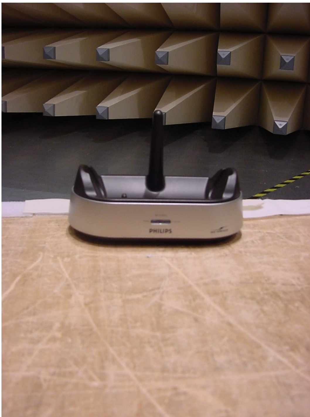
Photo 2 (Radiated Emissions): Tx Test set-up
