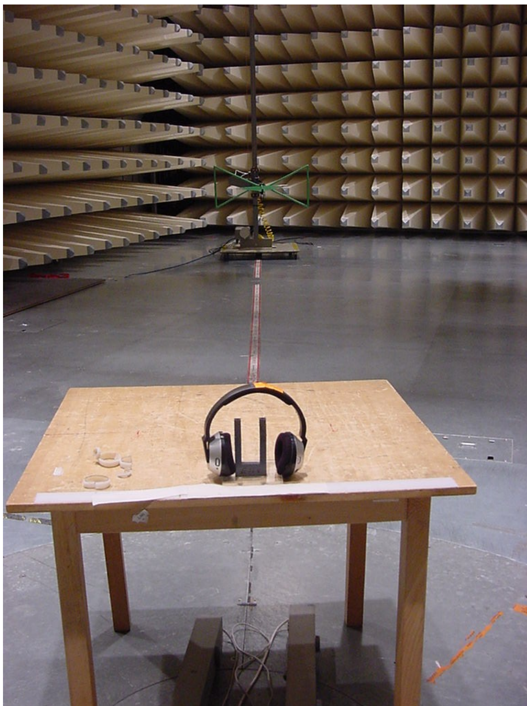
Photo 3 (Radiated Emissions): Rx Test set-up
