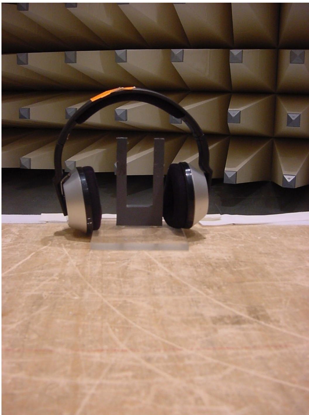
Photo 4 (Radiated Emissions): Rx Test set-up
