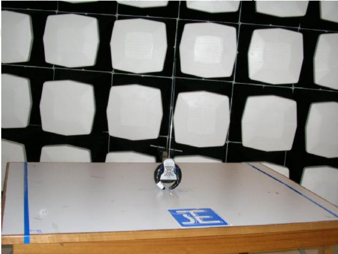
Measurement of Radiated Emission Test Set Up
