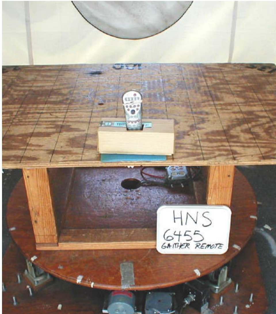
Figure 6: Radiated Emission Test Configuration, Z-Axis
