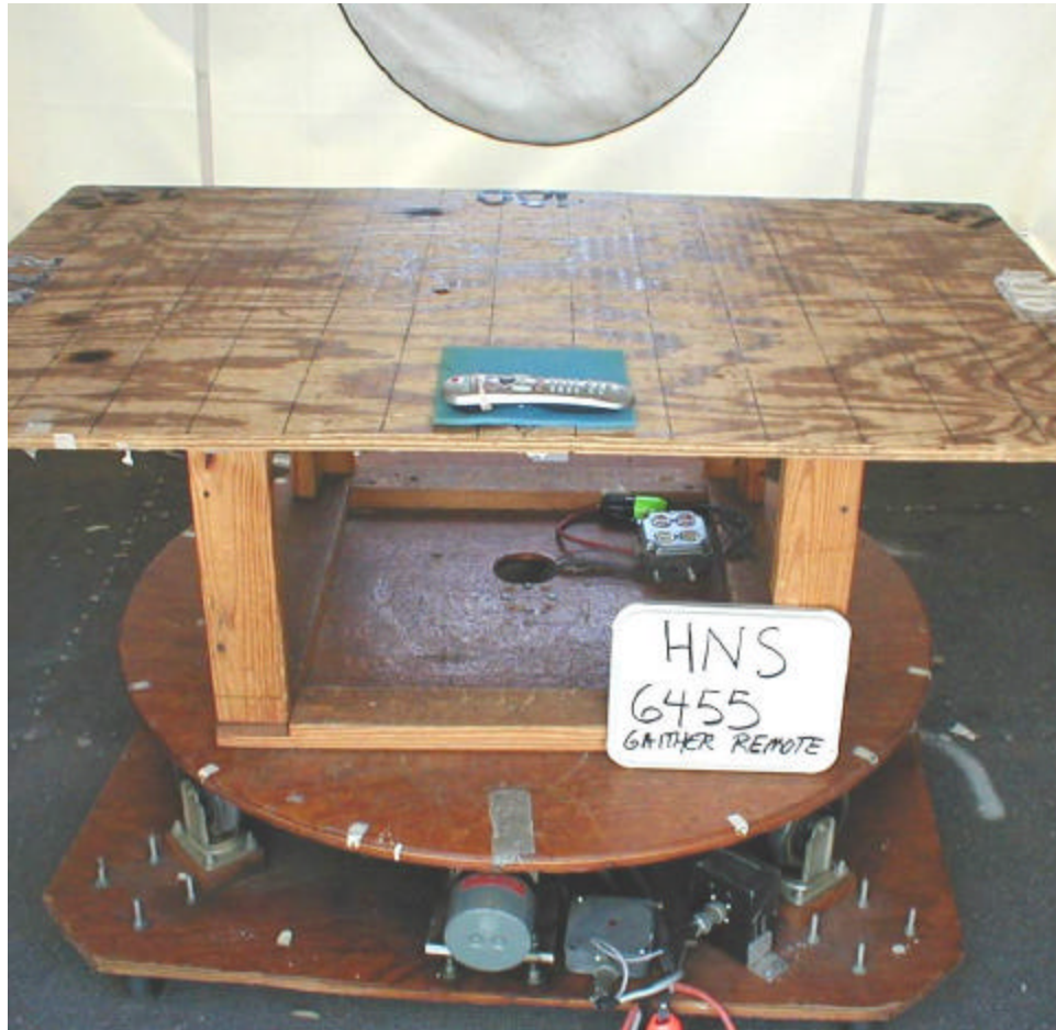
Figure 5: Radiated Emission Test Configuration, Y-Axis
