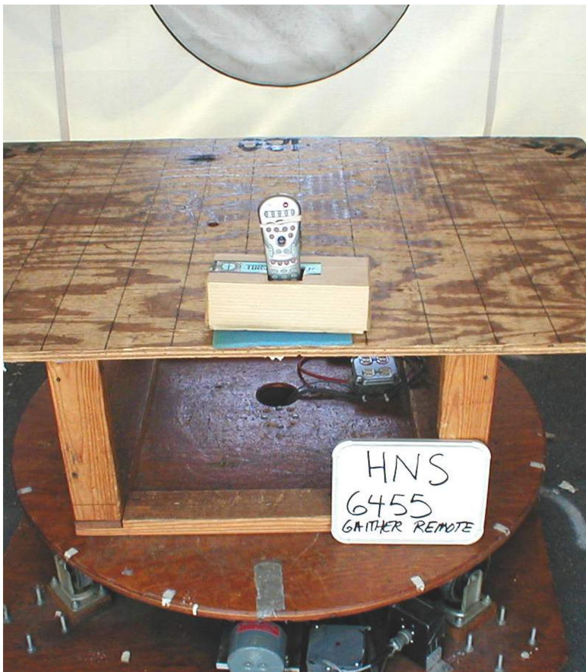
Radiated Emissions Test Setup, Vertical
