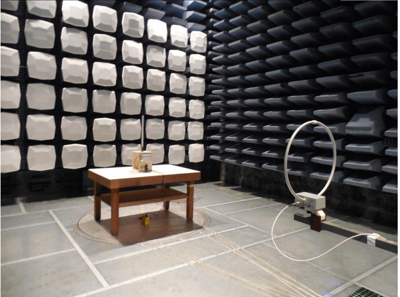
Figure 48: Emissions Test Setup – Intentional / Unintentional Radiated Emissions
