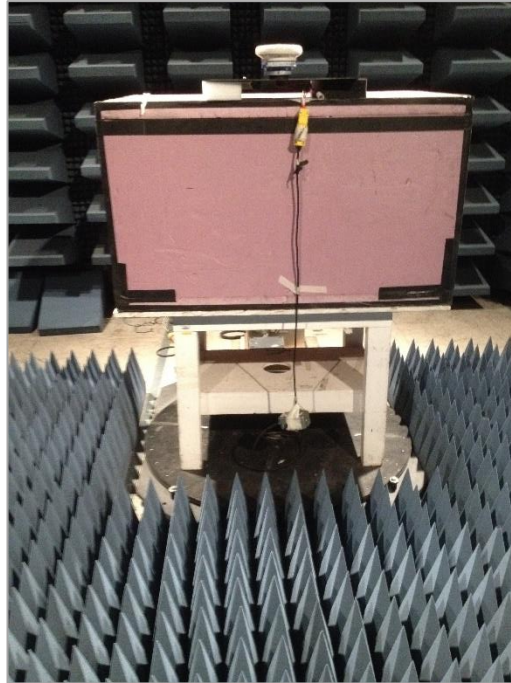
Figure 3: Radiated Emissions (close-up view) Test Setup
