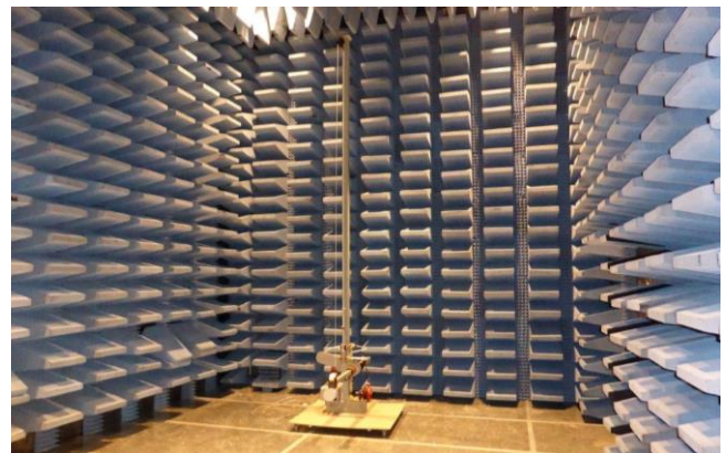
5 m Semi-Anechoic Chamber (SAC) in Everett, Washington
