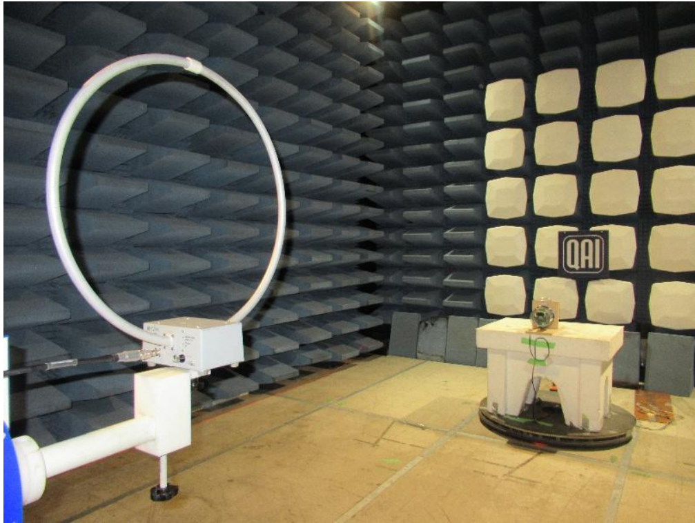
Figure 75: Radiated Measurement Setup, < 30 MHz
