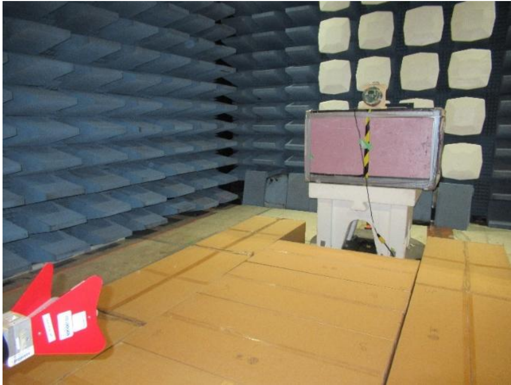
Figure 77: Radiated Measurement Setup, > 1 GHz
